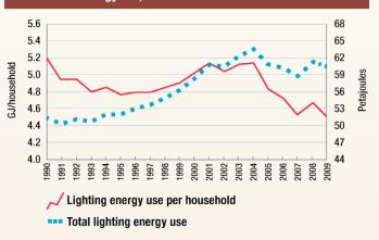
Some of the decrease in lighting energy use per household can be associated with the increased use of compact fluorescent lamps (CFLs), also known as compact fluorescent light bulbs (Figure 3.12), which use less energy to produce a certain level of light. The use of CFLs was marginal in the residential lighting market before 2000, but CFLs represented around 24 percent of light bulbs used in 2009.
